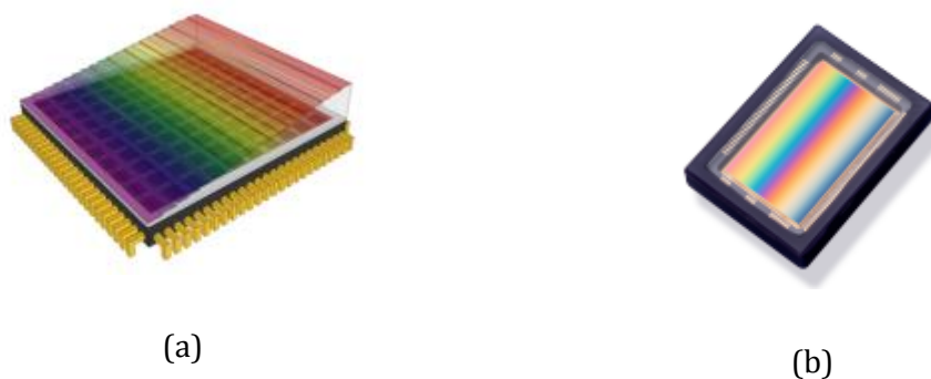
Figure 4: (a) concept of wedge layout (filter heights exaggerated for illustration) (b) a packaged wedge based hyperspectral imager
